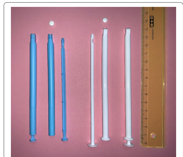
Fig. 1 Originator product (left) and newly developed product (right), both applicators consisting of a tube and a plunger
