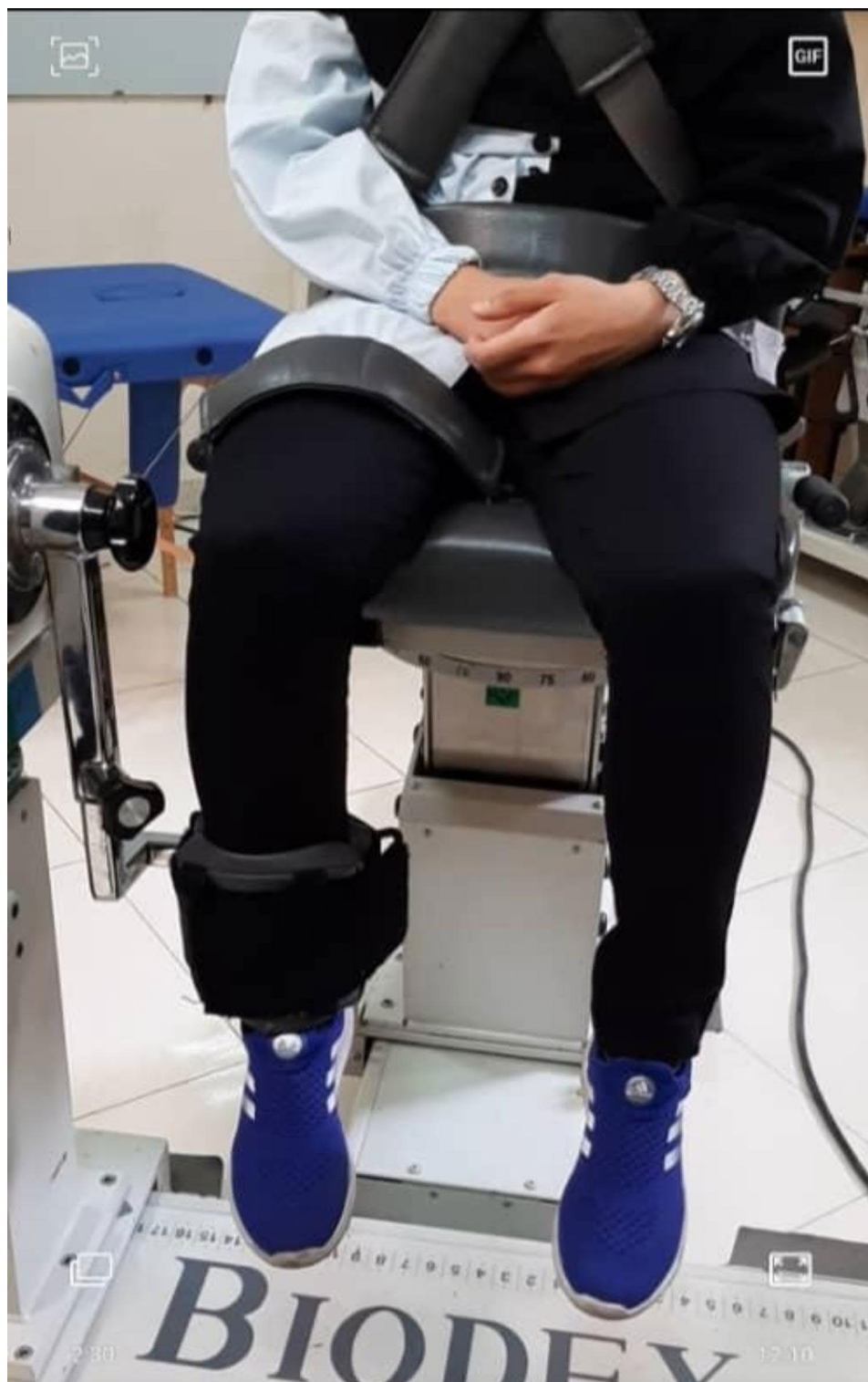
Fig. 1 Measurement of knee flexor and extensor muscle strength by using the isokinetic instrument
